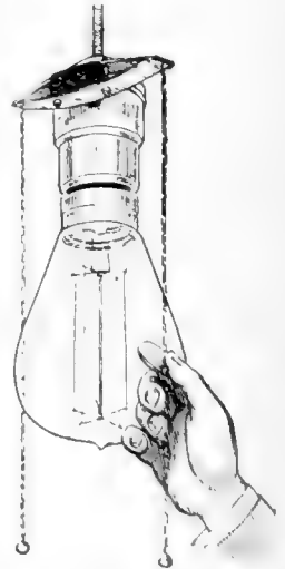
A pull-socket made from a key-socket
